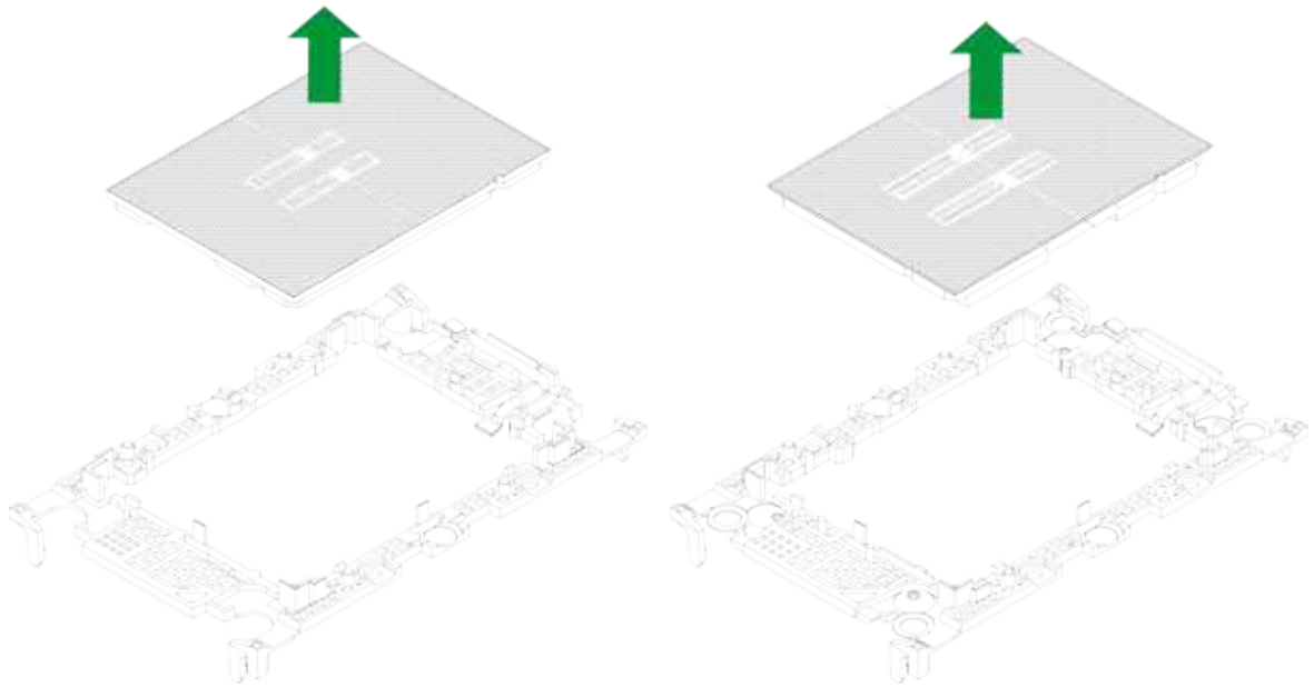
Figure 2-48. Removing the Processor (SP XCC left, SP HCC/LCC right)
